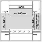
This distance should be increased to 700 mm if the wall cabinets are flammable (*see figure*).
